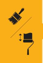
Apply the last stroke in one direction to ensure a uniform finish.
